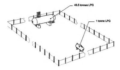
The small tank = 2% of medium hazard threshold (50 tonnes), but the separation from the large tank is sufficient to prevent the small tank starting a major incident at the large tank. It can therefore be ignored in terms of the 2% rule.
