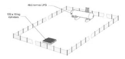
The separation between the compound and the large tank is sufficient to prevent the cylinders starting a major incident at the large tank.
