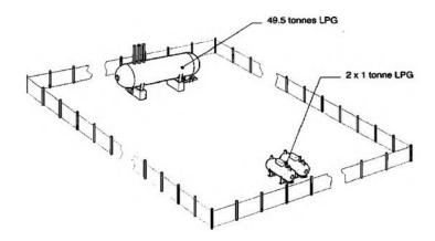
Each small tank = 2% of medium hazard threshold (50 tonnes), but their separation from the large tank and from each other is sufficient to prevent either of them starting a major incident at the other small tank or the large tank. Therefore, each can be ignored in terms of the 2% rule.
